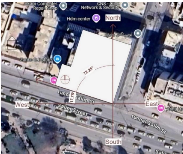
Figure 0-7 Building orientation showing the glazed façade aligned along the west-northwest axis ( 72.25^\circ from north (Source: Google Map).
