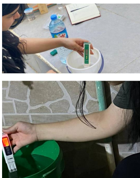
Figure 8: analyzing for hydrogen ion concentration (pH), temperature ( T^\circ\text{C} ), and electrical conductivity (EC) (Source: Authors).
